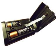
We use 2 batteries:- one for the transmitter, (AA or MN1500 size, 1.5V) and a separate battery just for the Laser (CR2, 3V). This is a high power/high capacity battery that is common in photographic systems and readily available.
